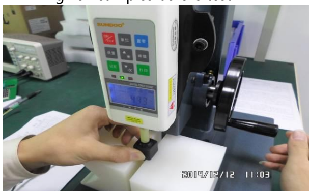
图 193 应力作用在镜头表面 Fig 193 strain applied on the surface of lens
