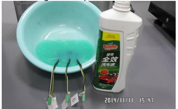
图 224 样品浸泡在溶液中 Fig224 samples immerse in the test liquid
