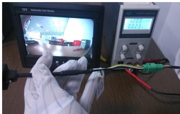
图 324 样品试验后通电 12V Fig324 samples apply with 12V after test
