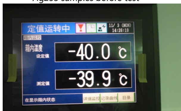
图 255 测试温度为-40°C Fig255 test temperature at -40°C
