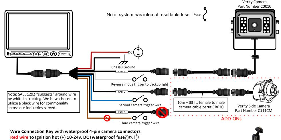
Red wire to Ignition hot (+) 10-24v. DC (waterproof fuse?) DC Black wire to GND. (-) White trigger for camera 1 / Black 4-pin (Cam 1) -Camera 1 Rear O O Blue trigger for camera 2 / Black 4-pin (Cam 2) – Optional Camera O O Brown trigger for camera 3 / Black 4-pin (Cam 3) Optional Camera O O
